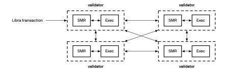
Figure 1: Integration of the SMR module into the Libra Blockchain
