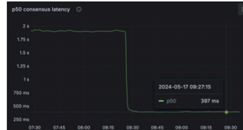
Fig. 1: P50 latency of a major blockchain switching from Bullshark (1900ms) to MYSTICETI-C (990ms) consensus on 106 independently run validators
